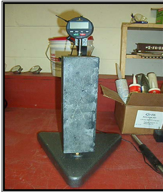
Figure 3: Shrinkage test setup and digital length comparator
